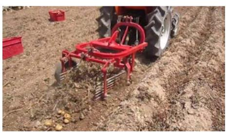
Potatoes are root vegetables, which means that harvesting them requires a lot of digging. The machine above tills the dirt around the potatoes and brings them up out of the ground. Even though the video depicts a small-scale machine, the same technology is used in tractor-towed rigs to harvest potatoes at an even greater scale.
