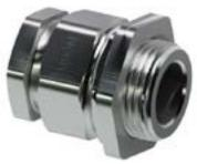
two knock-out hole sizes, namely 20 mm and 25 mm. While the nipple will pass through the 20 mm knock-out, the spigot will also fit a 25 mm hole. This is important because when fitting an ordinary 20 mm gland to a 25 mm hole, the gland tends to shift to one side and very often a corner of the lock nut slips into the hole. The worker fitting the gland becomes impatient, decides that the gland is tight enough and thereby compromises the earth continuity
